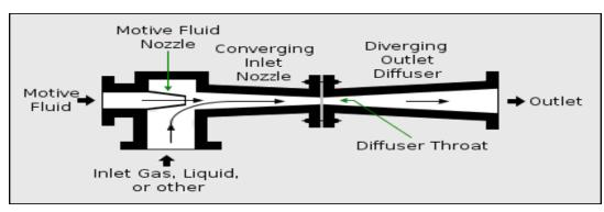
► The theory is that the speed (with that the moving energy) of the steam entering the converging nozzle will increase due to converging. The increased moving energy is balanced by decreased pressure. The pressure in the space around the nozzle will decrease so gas will be sucked into the nozzle from the surrounding space. In the diverging diffuser the moving energy will decrease and the pressure will increase again.
