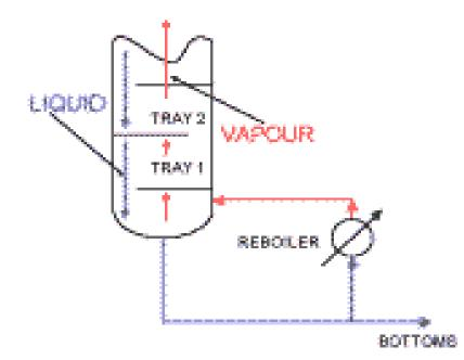
The liquid feed is flowing downwards and accumulates in the column bottom and reboiler.
