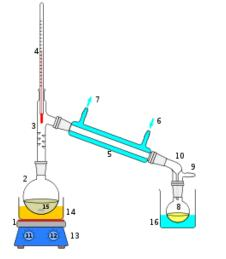
► The essence of distillation is to heat a given liquid until it became vapour and then condensing the vapours the material is converted to liquid again. Since there is no chemical alteration in the material structure, only phase transition, **the distillation is a physical process**.
