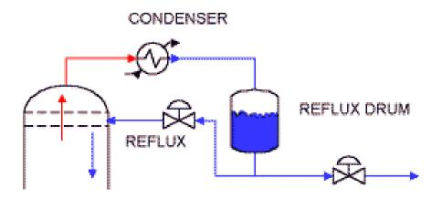
► The vapour flows upwards, and leaves the column at the top and reaches the condenser.
