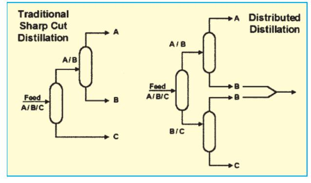
► The theory of distributed distillation is to minimize the number of sharp cuts. In the traditional sequence, the separation is done according to the relative volatility of the key components. Separation of components A, B and C in two columns will not utilize the distribution of B in the first column.
