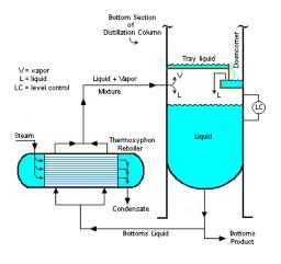
Thermosyphon reboiler (vertical)
