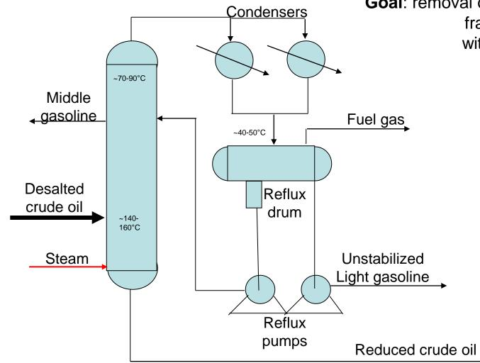
**Goal**: removal of lighter hydrocarbon fractions from crude oil, without direct heat input
