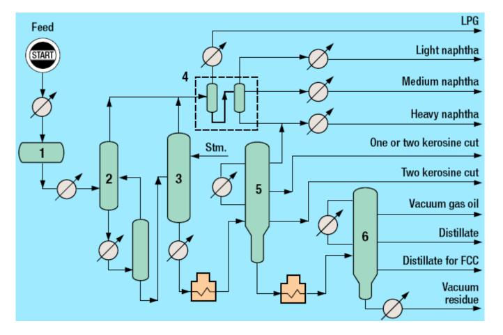
The Technip process was optimized for the following scheme: three gasoline, one/two petroleum, two atmospheric gasoil, one LVGO, two HVGO and vacuum residue cuts.
